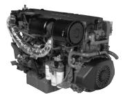
6-cylinder, 4-stroke, direct-injected, turbo-charged, and aftercooled marine diesel engine. Bore x Stroke (mm): 144 x 165
