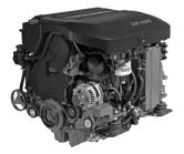
5-cylinder, 4-stroke, direct-injected turbo-charged, and aftercooled marine diesel engine. Bore x Stroke (mm): 81 x 93 Displacement (I): 2.4
