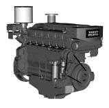
6-cylinder, 4-stroke, direct-injected, turbo-charged, and aftercooled marine diesel engine. Bore x Stroke (mm): 108 x 130 Displacement (I): 7.15 6-cylinder, 4 stroke, direct-injected, common rail, turbo-charged, and aftercooled marine diesel engine. Bore x Stroke (mm): 110 x 135 Displacement (I): 7,7
