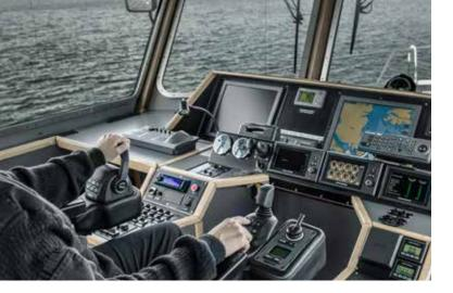
The buttons on the joystick put a unique combination of functions within your easy reach. Dynamic Positioning, Joystick Driving, Joystick Docking and High Mode offer easier handling, increased safety, and reliable operation.
