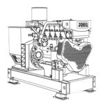
4-cylinder, 4-stroke, direct-injected, and turbo-charged aftercooled marine diesel engine. Bore x Stroke (mm): 108 x 130 Displacement (I): 4.76 6-cylinder, 4-stroke, direct-injected, and turbo-charged marine diesel engine. Bore x Stroke (mm): 108 x 130 Displacement (I): 7.15
