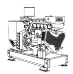
4-cylinder, 4-stroke, direct-injected, and turbo-charged marine diesel engine.
